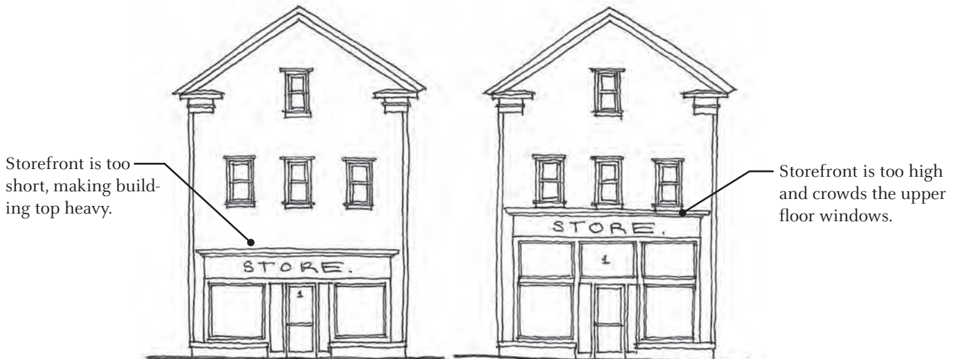
Poorly proportioned buildings result when either of the mixed-use functions are not of the appropriate scale.
